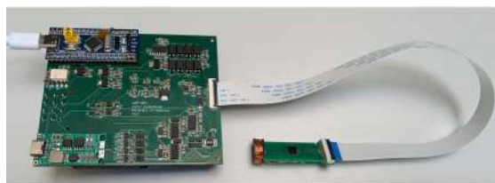
Figure 1: The standalone, compact electronics module (left) and the sensor head (right), which is composed of two magnetoresistive sensors and the excitation coil.
